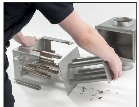
The large stripper plate guarantees quick and safe cleaning.
